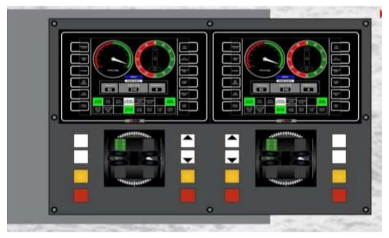
The Azimuth Thruster Control System (ACS) fully automates from bridge the control of the electric azimuth thruster systems through the VFD or AFE drive control and provides full 360 degree control with full feedback (closed loop) units.
