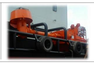
Deck Mounted – Direct Engine Drives complete with Diesel Engine, Clutch and Azimuthing and Retractable Drive
