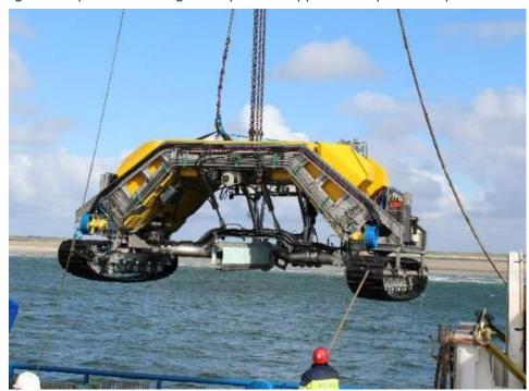
The thruster systems are pressure compensated and operational to all ocean depths.
