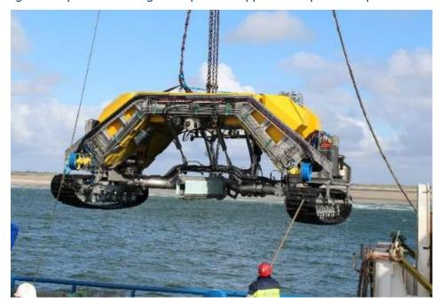
The thruster systems are pressure compensated and operational to all ocean depths.
