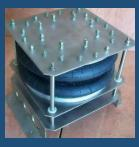
The 18L style unit is of SS316 construction and comes with double convoluted diaphragm. This design is available in 18 to 33L volumes with double or triple convoluted diaphragms, depending upon volume required. Ports arrangements & gty are to user requirement.
